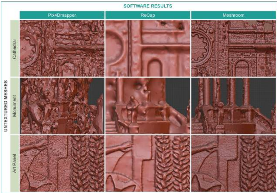
Figure 6: Details of the three captured elements in the different software without texture.
