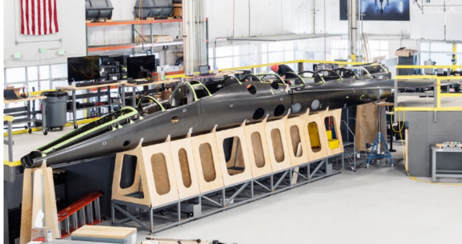
Figure 1.2 – XB-1 prototype aircraft with fuselage and wings assembled.
