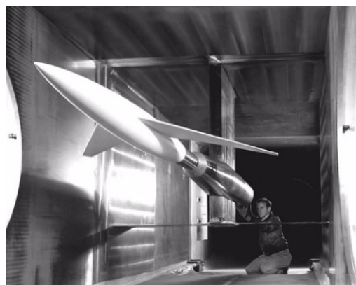
(b) Test section with large scale model.
