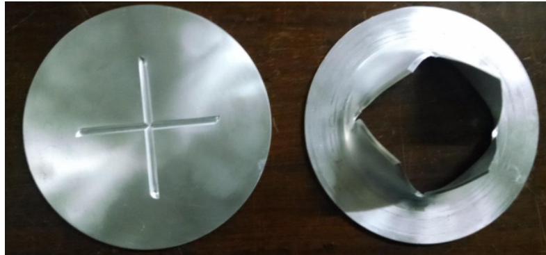
Figure 3.9 – Prepared grooved diaphragm (left) and burst diaphragm after test run (right).
