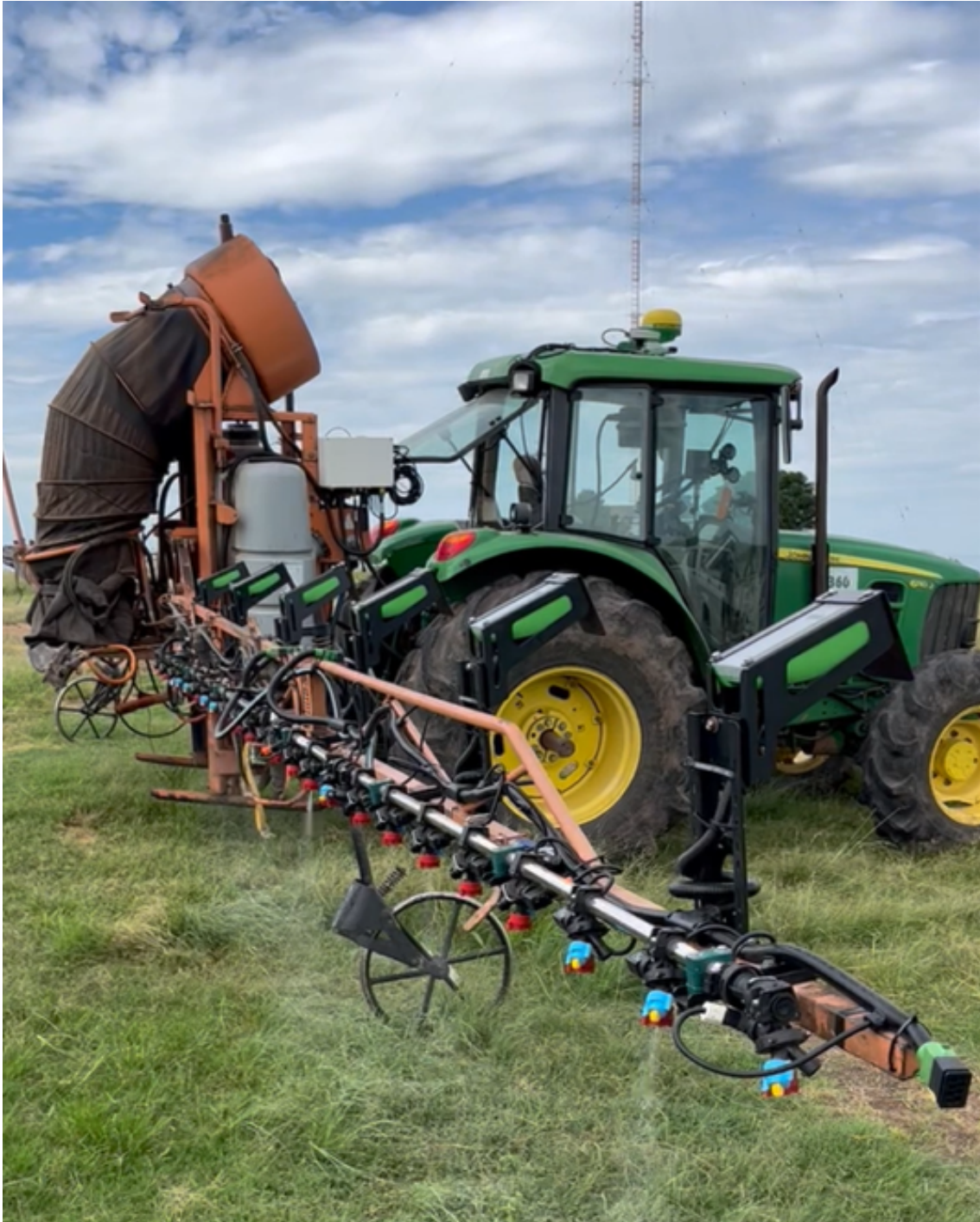
Figure 2: Sprayer (6m boom) being tested with the Weed-IT mounted on it.
