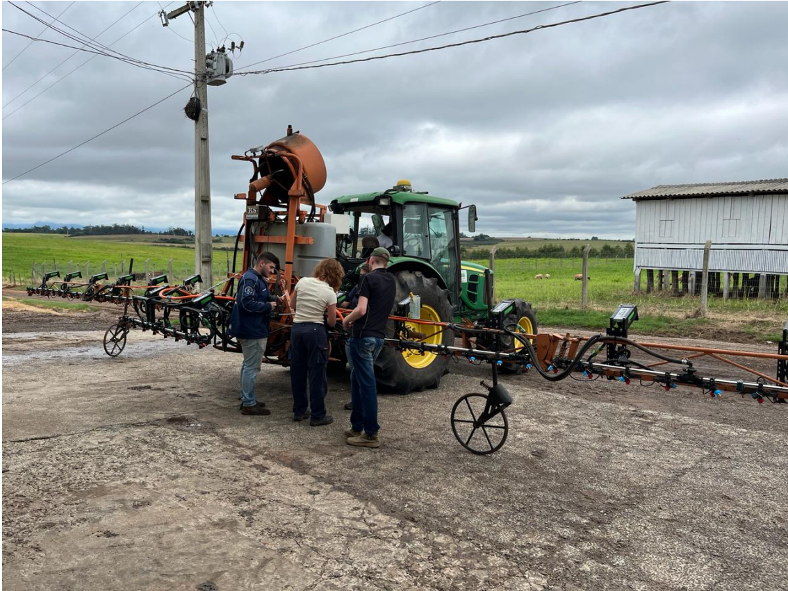
Figure 2: Sprayer (6m boom) being tested with the WEED-IT mounted on it.
