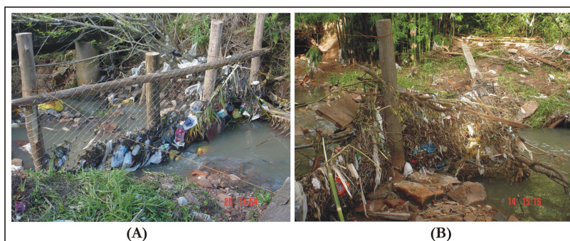
Figure 6 – Collector nets with the retained material after a rainfall event at Alto da Colina (A) and Cancela (B) stations
