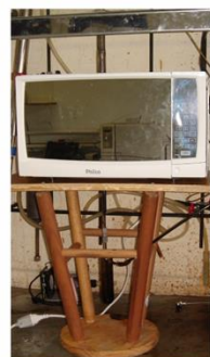
pyrolysis of organic precursor assisted by microwaves. Releases of gases during the pyrolysis.
