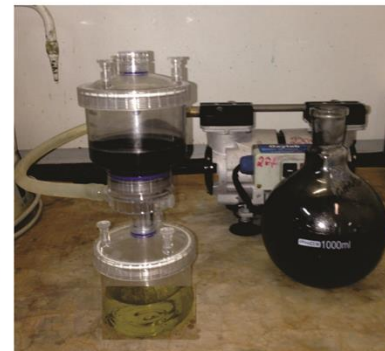
Activation step: Lixivation of inorganics and filtration
