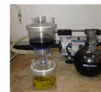
filtration of activated carbon
