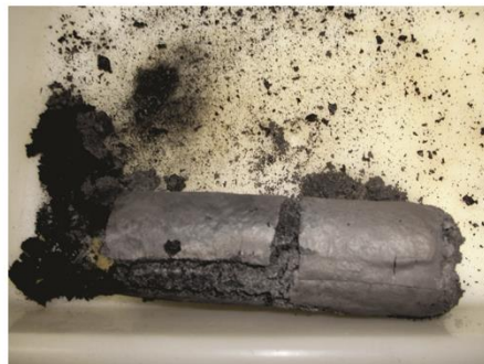
carbon material removed in cylinder form out of reactor
