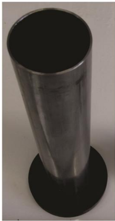
Cylinder for preparation of activated carbon
