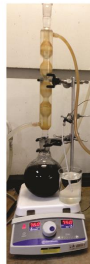
Activation step: Lixivation of inorganics and filtration
