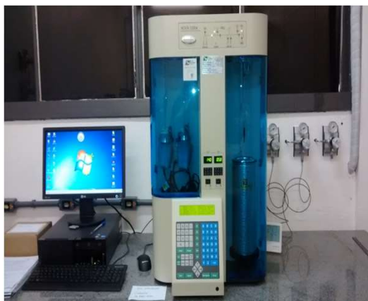
Surface Area Analyser Quantachrome/NOVA1200E
