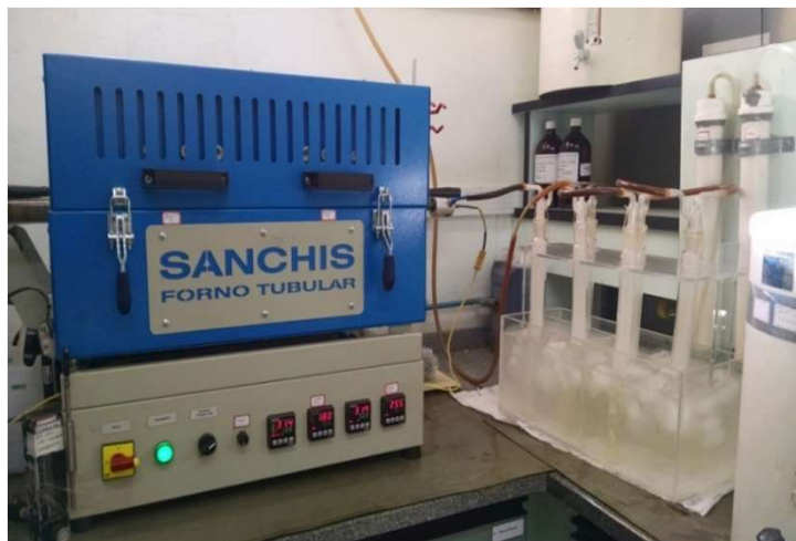
Fixed-bed/Rotative reactor Application: Pyrolysis/gasification reactions. Biomass and waste combustion.
