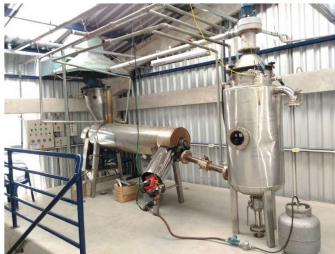
Screw reactor Application: Pyrolysis reactions. Biomass and waste.
