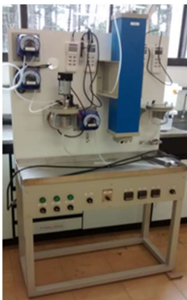
Multipurpose reactor (CSTR/PFR) Application: Catalytic homogeneous/heterogeneous reactions. Production of biodiesel.
