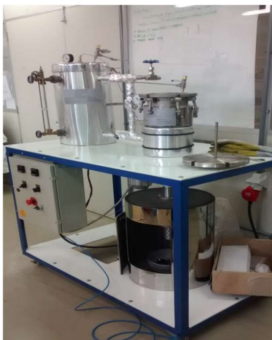
Steam explosion reactor Application: Separation of biomass fibres and lignin removal
