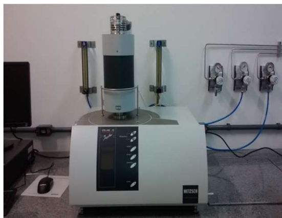
Thermogravimetric Analyser TG/DSC NETZSCH STA449F3 Jupiter.
