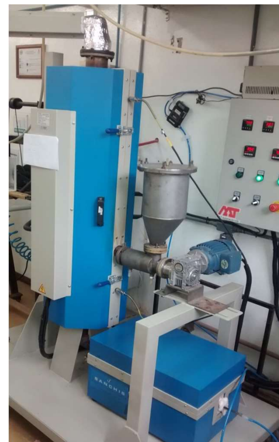
Fixed or Fluidized-bed reactor Application: Pyrolysis/gasification reactions. Biomass and waste combustion.
