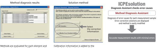
Methods are evaluated for each element and each sample. If there are differences from the analysis values, the problem point is indicated. Calibration information is added to the method simply by selecting the solution method in the sequence shown. Method is automatically modified.
